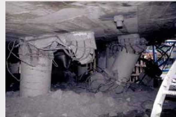
Failure of concrete piles supporting Liquid oxygen tanks during the 1999 Izmit earthquake in Turkey
