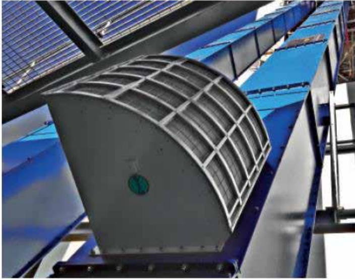
Explosion Safety of a trough chain conveyor using the Q-Box in a biomass power plant.
