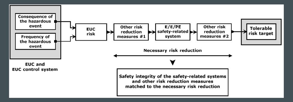
Measures # 1: e.g. BPCS;  $R_R < 10$ E/E/PES:  $10 \ge R_R < 10.000$ Measures # 2: Mitigation Systems (e.g. F&G Systems, Leakage monitoring etc.)
